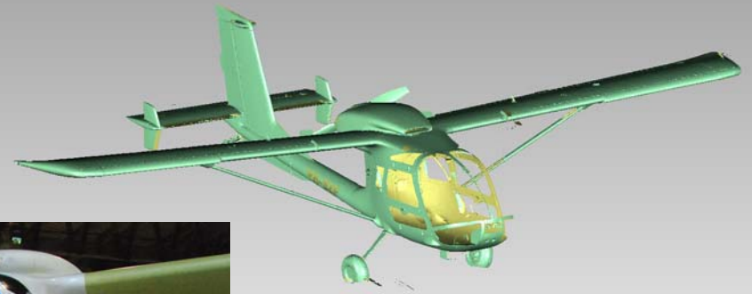
Scan data as Point Cloud
